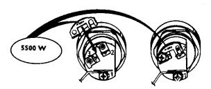
7. The wire removed from terminal 2 has a looped end. It must remain looped and now be placed (as shown) on top of the buss bar, over the opening of terminal 2, and secured using the remaining screw.
